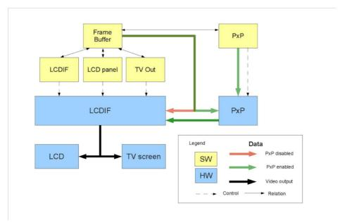
Figure 2-2. **i.MX28** Kernel Graphic Components
