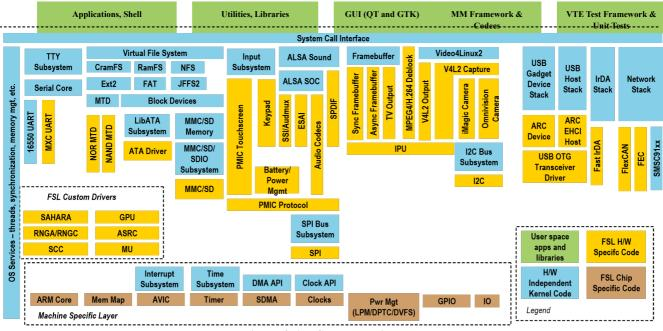
Figure 2-1. BSP Block Diagram
