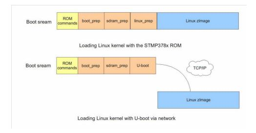
Figure 2-6 shows block diagrams of two boot stream images.
