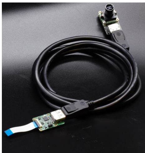
CSI2 MIPI REMOTE LVDS CABLE APPLICATION
