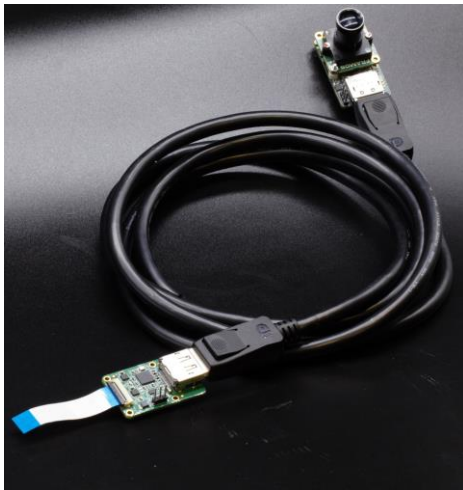
CSI2 MIPI REMOTE LVDS CABLE APPLICATION
